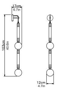
240V Illumination Integrated LED Lumens: 900Im Colour Temperature: 2700K Dimmable: LED dimmer required
